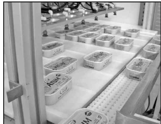
ACCUMULATION TABLES OF CONTAINERS
